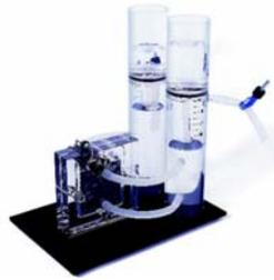
Figure 4 Small Home Appliance Electrolyzer (Fuel Cell Store, 2002)
